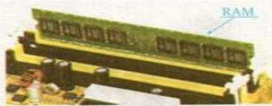
Fig. 1.1.3a RAM is plugged in a socket
